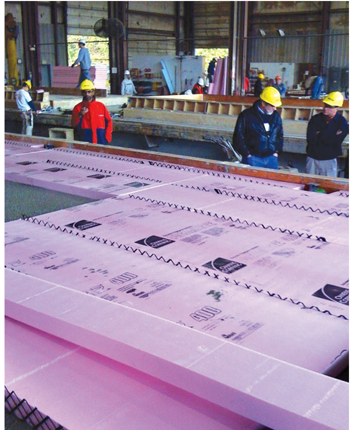
Right: Carbon fiber grid connectors and XPS insulation
