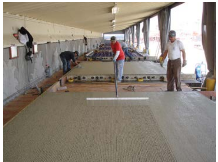
Figure 7.23. Commercially available rake being used to impart macrotexture on top of a previously applied burlap drag ("microtexture") finish. Source: Pro-Cast Products
