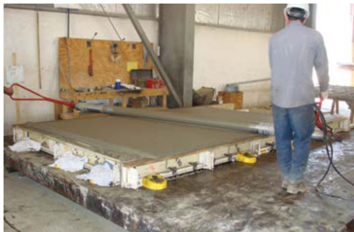
Figure 7.10. Magnetically anchored side rails being used on all four sides of a single-panel form. Source: The Fort Miller Co., Inc.
