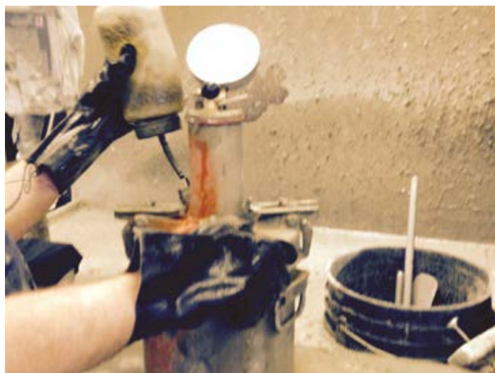
Figure 7.18. Standard ASTM slump test (left) and air content testing by the pressure method (right). Source: The Fort Miller Co., Inc.
