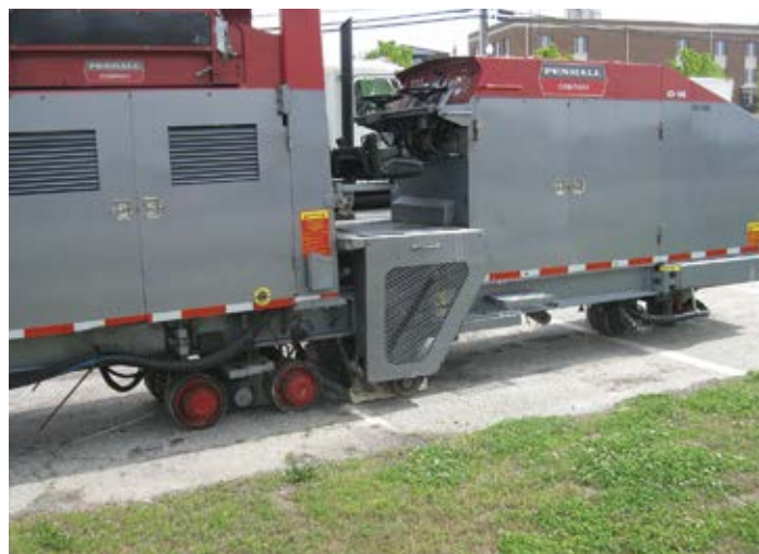
Figure 11.22. The bogie wheels on the left control the cross-slope of the head while the dual in-line center wheels on the right establish the longitudinal profile of the machine. Source: The Fort Miller Co., Inc.
