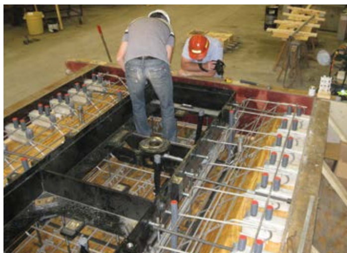
Figure 3.28. Frame for weigh-in-motion scales positioned in a precasting form. Source: The Fort Miller Co., Inc.
