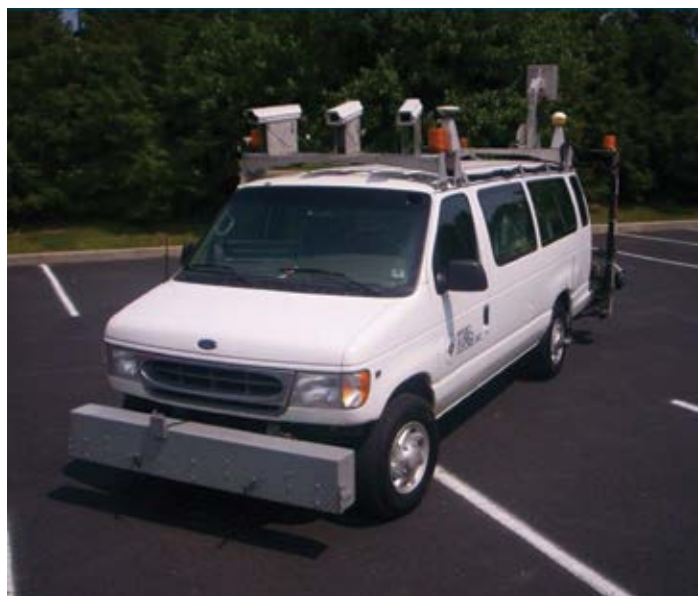
Figure 12.2. This digital survey vehicle gathers data while traveling at or near highway speeds. Source: Applied Research Associates, Inc.
