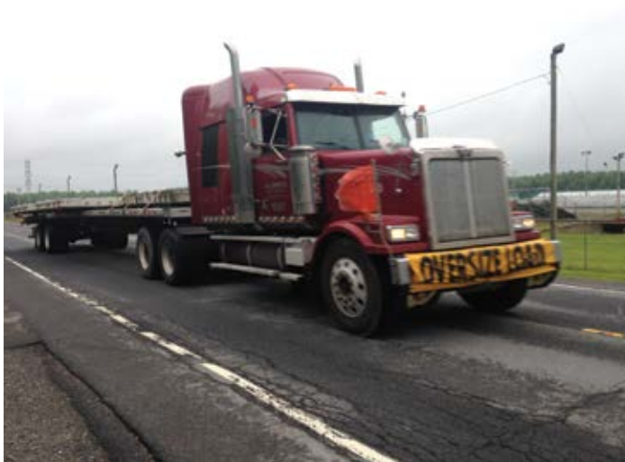
Figure 7.32. Example of vehicle signage for over-width loads (requirements vary by state). Source: The Fort Miller Co., Inc.
