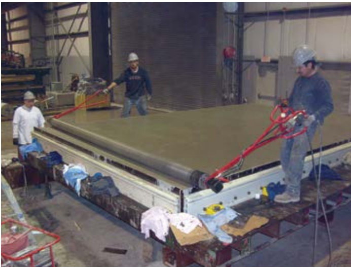
Figure 7.21. A hydraulically powered roller screed saves labor and time, producing a more accurate panel surface. Source: The Fort Miller Co., Inc.
