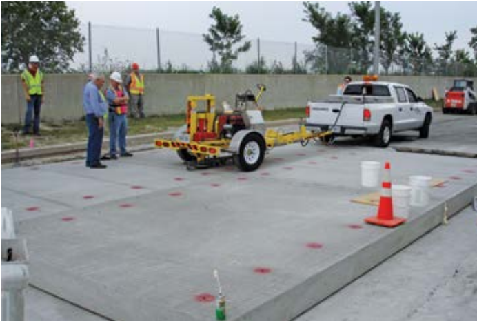
Figure 10.2. Falling weight deflectometer equipment measuring load transfer efficiency at a trial installation in Chicago, Ill. Source: The Fort Miller Co., Inc.
