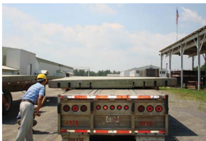
Figure 7.7. Warped-plane panel with a 4-inch delta (warp) on a truck. Source: The Fort Miller Co., Inc.
