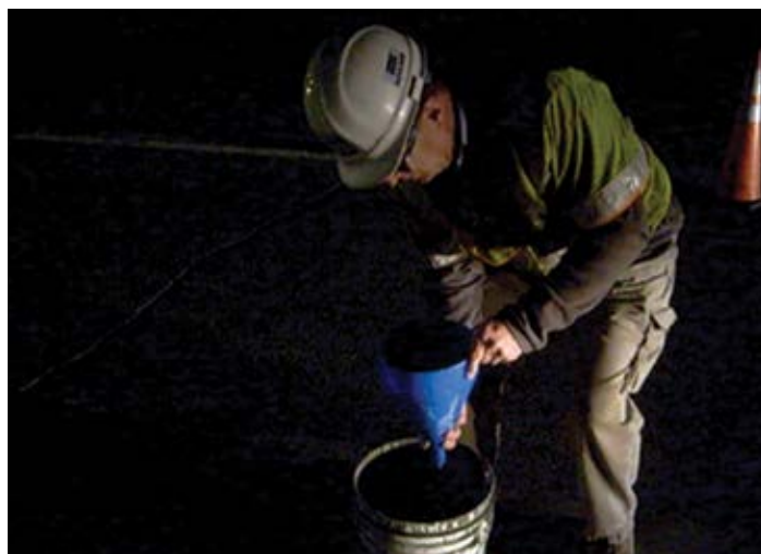
Figure 9.14. A worker performs a flow test in accordance with ASTM C939 to ensure proper consistency of the bedding grout. Source: The Fort Miller Co., Inc.
