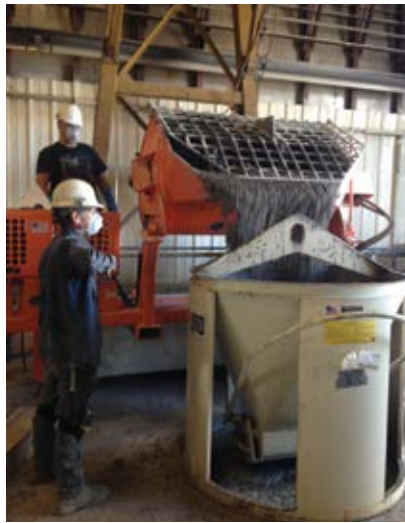
Figure 13.21. Mixed polymer concrete being discharged from a mixer into a concrete bucket. Source: The Fort Miller Co., Inc.
