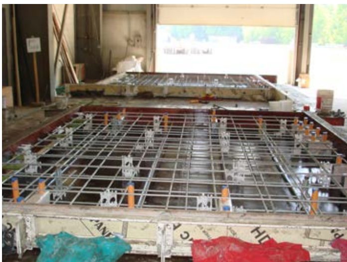
Figure 1.8. Two layers of reinforcing steel in each direction in a JPrCP fabrication. Source: The Fort Miller Co., Inc.
