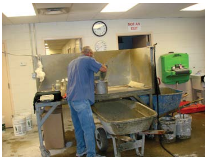
Figure 10.4. An American Concrete Institute-certified concrete technician measures air content. Source: The Fort Miller Co., Inc.
