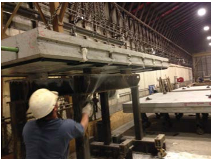
Figure 7.29. Application of sprayed curing compound to all panel surfaces. Source: The Fort Miller Co., Inc.
