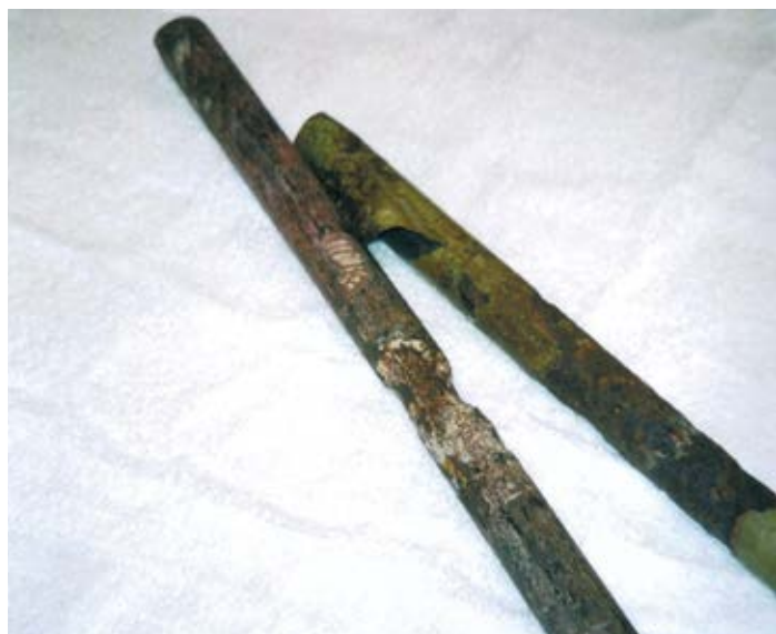
Figure 4.24. Dowels retrieved from Minnesota pavements after 17 years or more of service. Source: Doug Schwartz, Minnesota Department of Transportation
