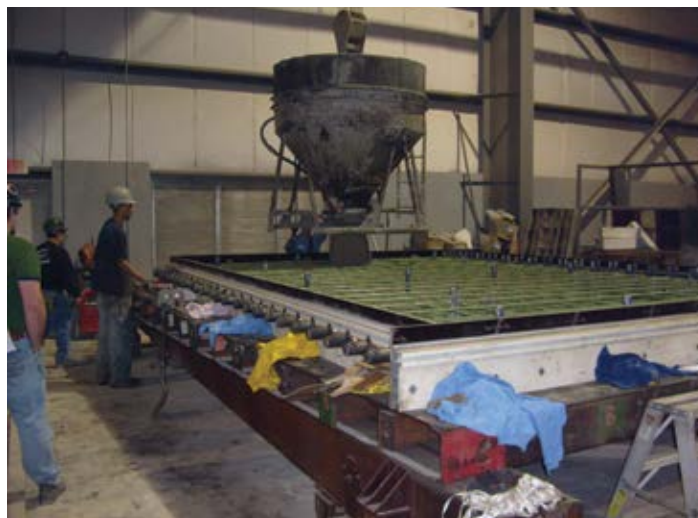
Figure 7.19. Use of a conventional concrete bucket to place panel concrete in a "high" form. Source: The Fort Miller Co., Inc.
