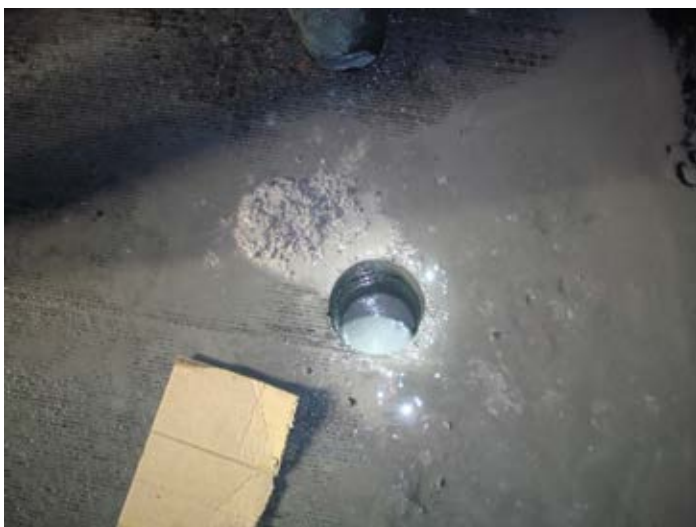
Figure 2.14. Water standing in a core hole several minutes after retrieval, indicating poor drainage of underlying layers. Source: The Fort Miller Co., Inc.
