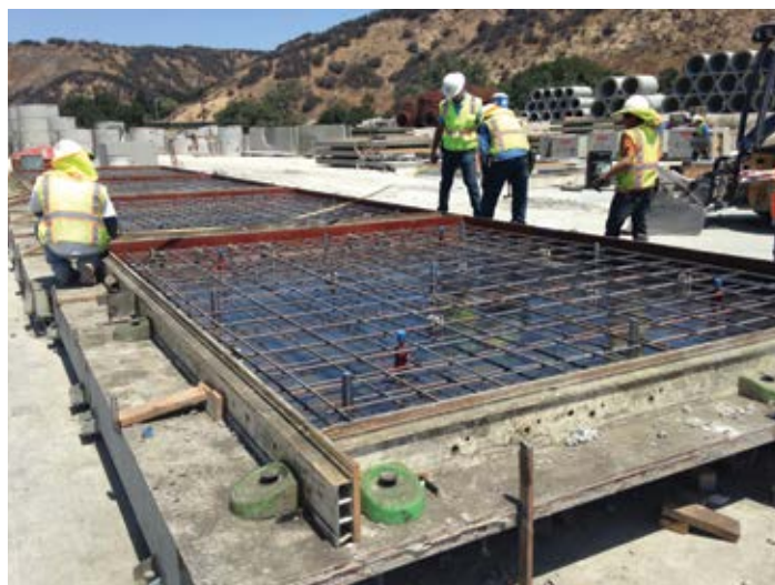
Figure 7.9. Aluminum extrusions (faced with special plywood) anchored with magnets in a long-line bed. Source: The Fort Miller Co., Inc.
