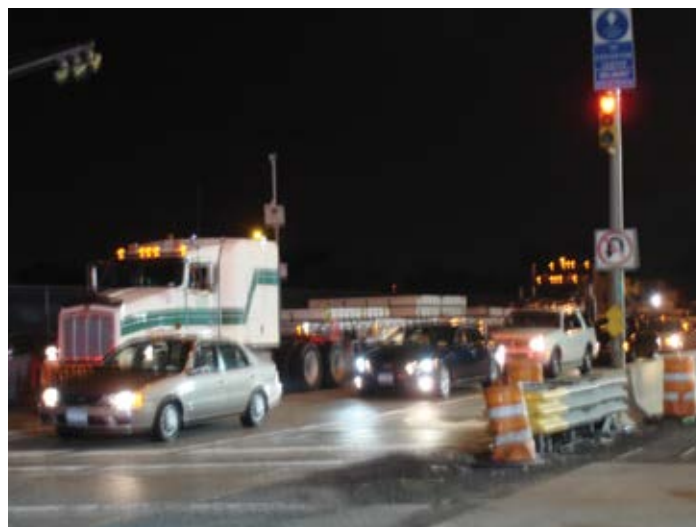
Figure 7.33. Ten-foot-wide (over-width) precast panels being shipped in New York City at night. Source: The Fort Miller Co., Inc.
