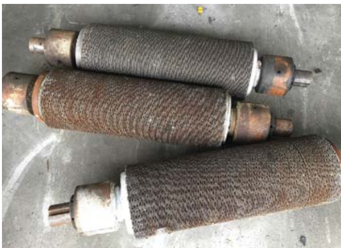
Figure 11.21. Closely spaced saw blades can be seen in this photo of a diamond profile grinding head. Source: Penhall Company
