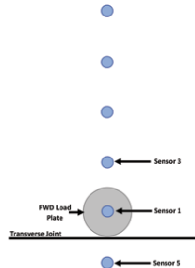
Figure 4.29. FWD sensor configuration example for Test Location 2 in Figure 4.27 (after Caltrans, 2015).
