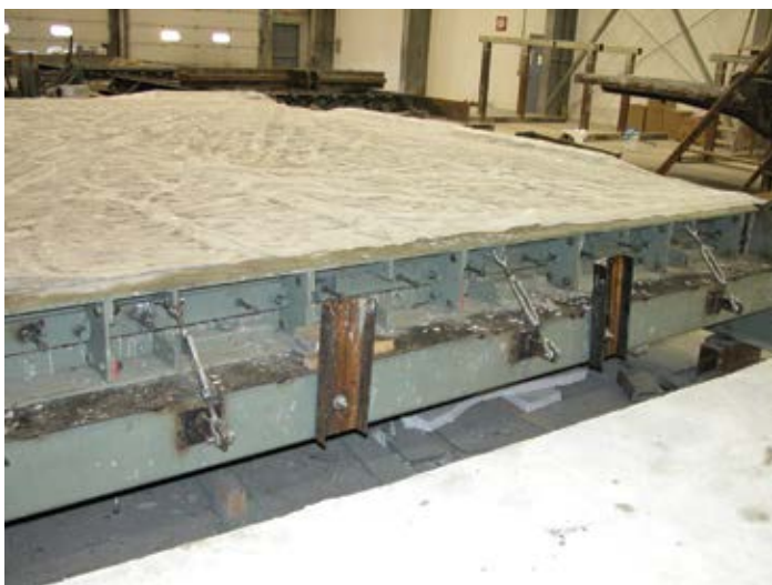
Figure 7.8. Turn buckles and push bolts are used to keep the tops of side rails straight. Source: The Fort Miller Co., Inc.
