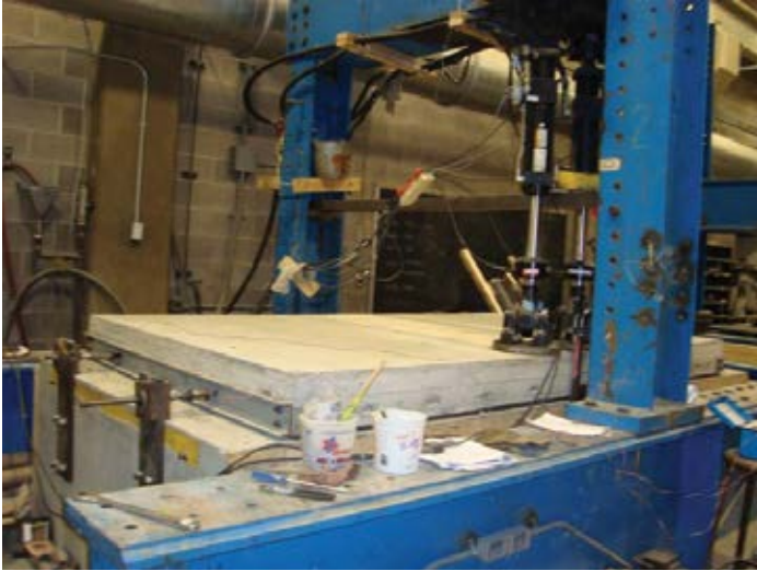
Figure 4.30. Photo and schematic of University of Pittsburgh lab-based accelerated loading pavement test stand. Source: J.M. Vandenbossche, University of Pittsburgh
