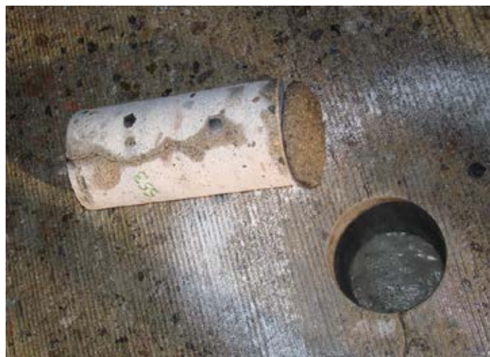
Figure 11.10. The crack in this core measured .06 inches wide at the top of the core and stopped at the bottom layer of reinforcing. Source: The Fort Miller Co., Inc.
