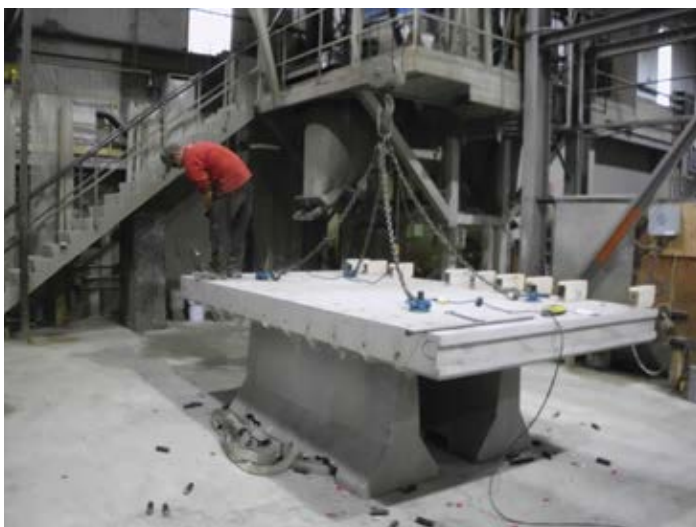
Figure 7.26. Panel placed on waist-high stands to facilitate stripping of slot formers, post-pour checking and panel detailing. Source: The Fort Miller Co., Inc.
