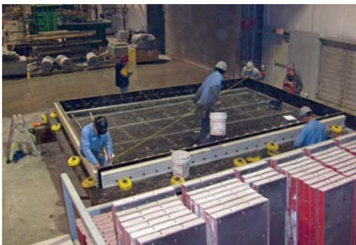
Figure 7.14. Checking form diagonals during form setup. Source: The Fort Miller Co., Inc.
