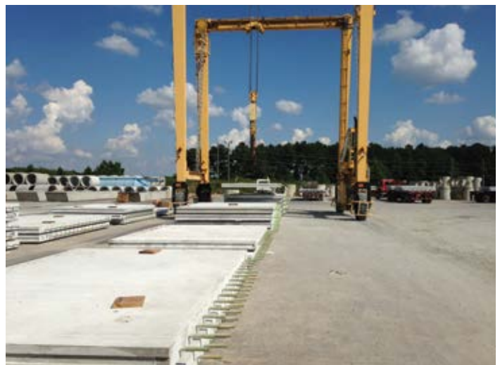
Figure 7.30. Illustrations of proper dunnage placement for panels in storage and for panels ready to be shipped. Source: The Fort Miller Co., Inc.
