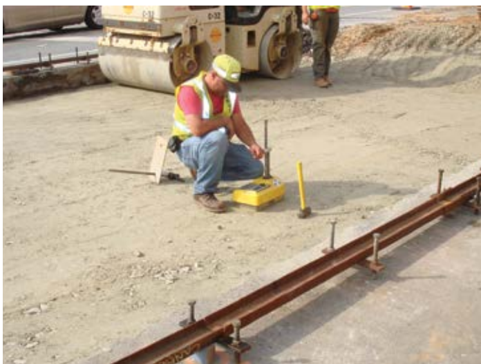
Figure 8.28. Density testing of newly placed subbase material to evaluate compaction. Source: The Fort Miller Co., Inc.
