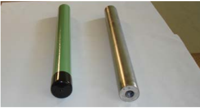
Figure 13.6 A flanged nut is welded to both ends of a tubular stainless steel Super-Dowel, shown at right. An epoxy-coated tubular carbon steel dowel, capped and ready for installation, is pictured on the left. Source: The Fort Miller Co., Inc.
