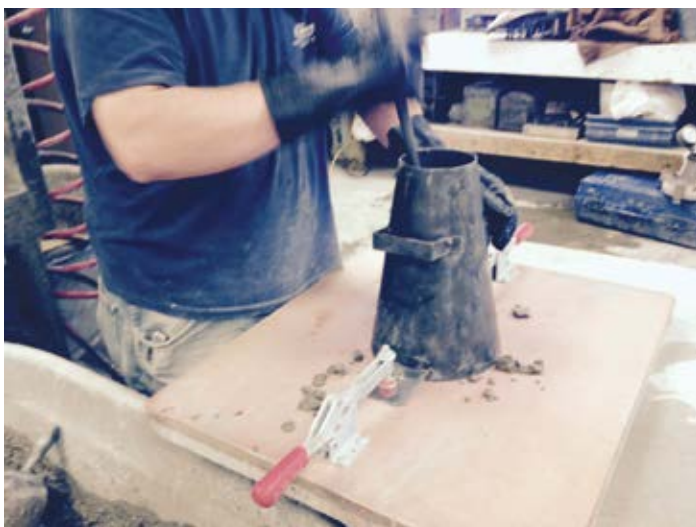
Figure 7.18. Standard ASTM slump test (left) and air content testing by the pressure method (right). Source: The Fort Miller Co., Inc.
