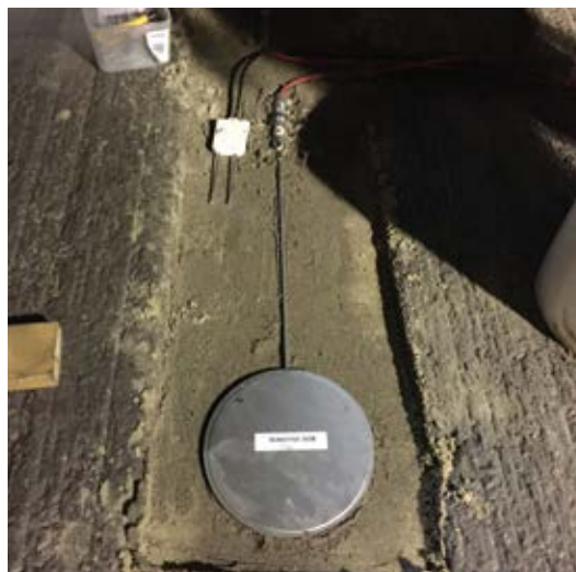
Figure 13.16. A moisture sensor and load cell being installed. Source: The Fort Miller Co., Inc.
