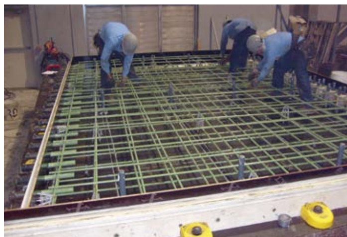
Figure 7.13. Adjustable side rails for producing general panels of any size or shape. Source: The Fort Miller Co., Inc.
