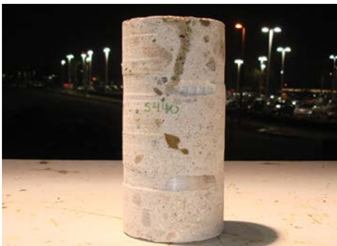
Figure 11.9. The shallow crack in this core, measuring approximately .02 inches wide at the top of the panel, stopped at the top layer of reinforcing. Source: The Fort Miller Co., Inc.
