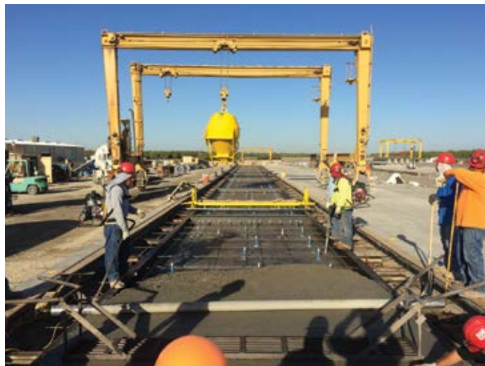
Figure 7.4. Long-line prestressing beds with adjustable end rails. Source: Con-Fab California, LLC
