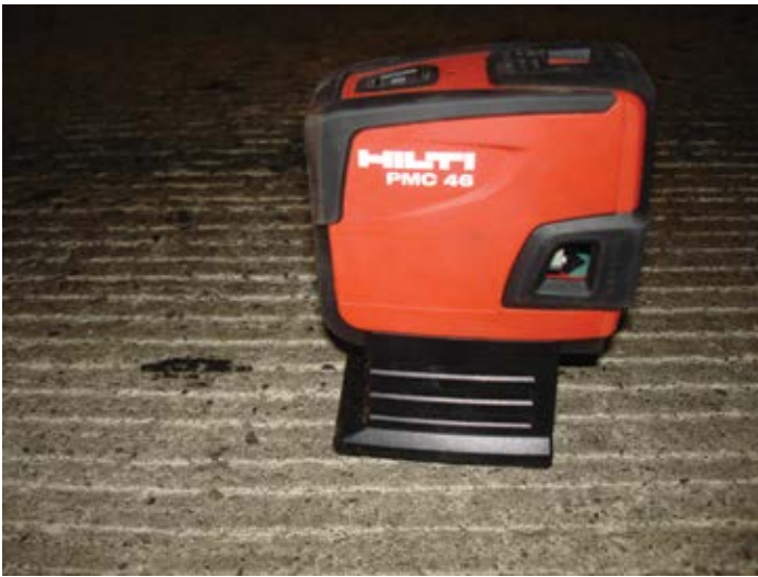
Figure 8.9. An example right-angle laser device for laying out perpendicular transverse saw cut lines. Source: The Fort Miller Co., Inc.
