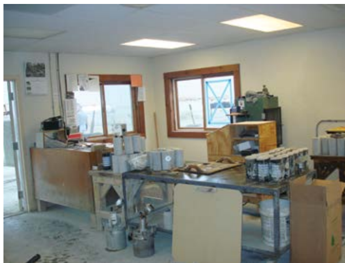
Figure 10.3. Entrained air meter and compression testing equipment in a precast plant testing lab. Source: The Fort Miller Co., Inc.
