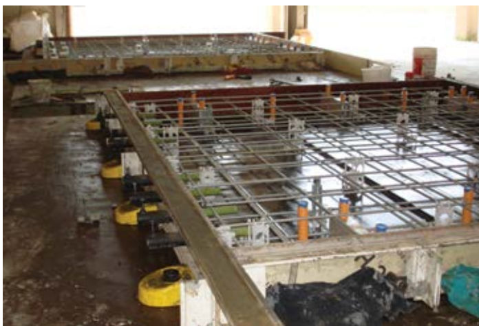
Figure 7.16. Typical placement of lifting inserts and rebar chairs. Source: The Fort Miller Co., Inc.
