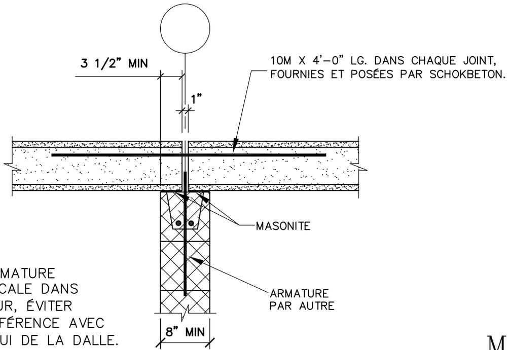
NOTE: SI ARMATURE VERTICALE DANS LE MUR, ÉVITER INTERFÉRENCE AVEC L'APPUI DE LA DALLE.
