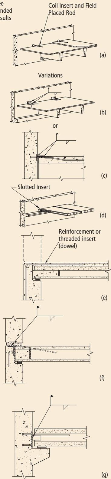
Fig. 4.5.76 Slab to bearing wall (SBW2).
