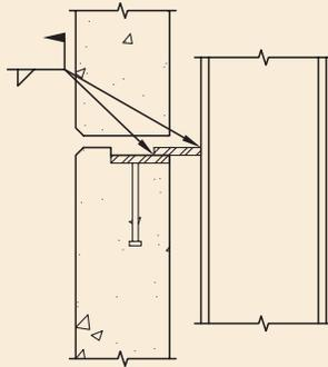
Fig. 4.5.33 Welded tieback (WTB5).
