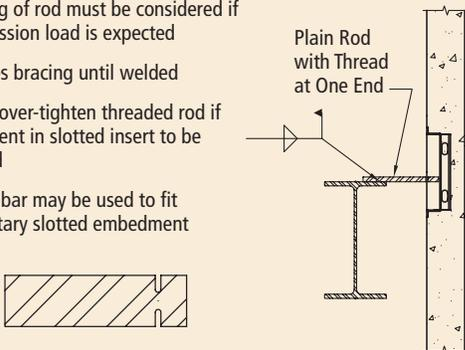
Fig. 4.5.34 Welded tieback (WTB6).
