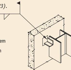
Fig. 4.5.48 Shear plate (SP4).
