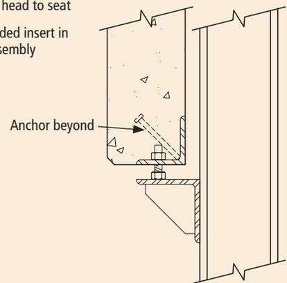
Fig. 4.5.23 Eccentric bearing (EB1).
