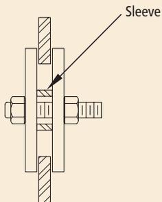
(c) Small diameter tieback rods desired for flexing can be prevented from buckling in compression with loose pipe sleeve
