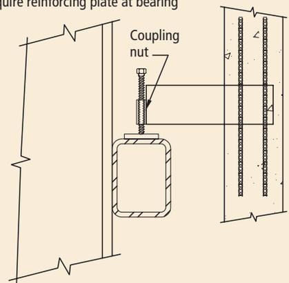
Fig. 4.5.29 Welded tieback (WTB1).
