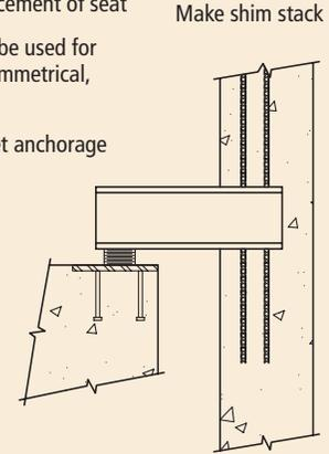
Fig. 4.5.24 Eccentric bearing (EB2).
