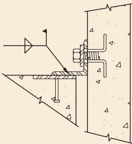
Fig. 4.5.39 Bolted tieback (BTB3).
