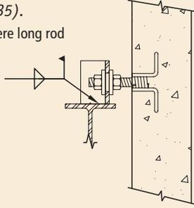
Fig. 4.5.42 Bolted tieback (BTB6).
