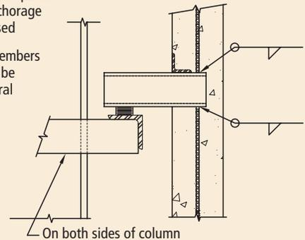
Fig. 4.5.25 Eccentric bearing (EB3).
