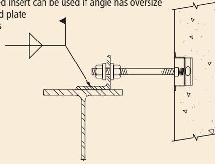
Fig. 4.5.36 Welded tieback (WTB8).
