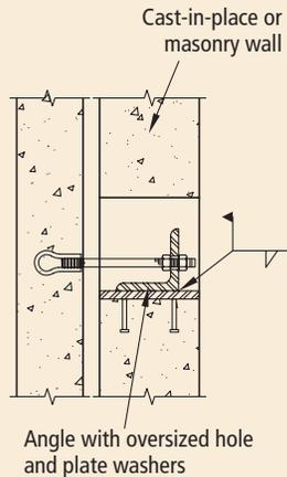
Fig. 4.5.45 Shear plate (SP1).
