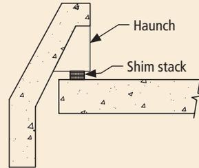
Fig. 4.5.18 Direct bearing (DB4).
