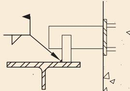
(b) Use in pairs. Round bars shop welded to bearing bracket.
