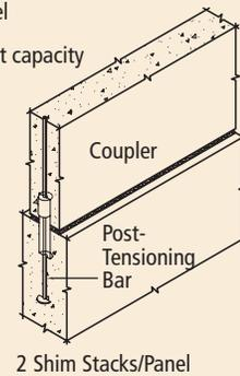
Fig. 4.5.75 Slab to bearing wall (SBW1).
