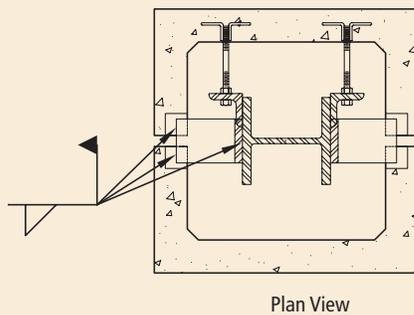
Fig. 4.5.63 Soffit hanger (SH1).
