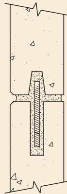
Fig. 4.5.21 Direct bearing (DB7).
