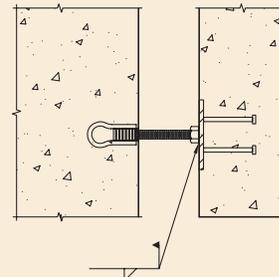
Fig. 4.5.35 Welded tieback (WTB7).
