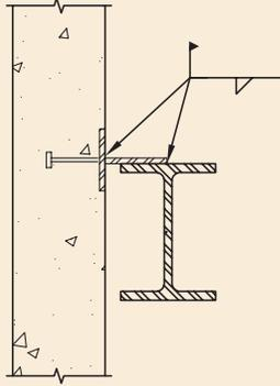
Fig. 4.5.32 Welded tieback (WTB4).
