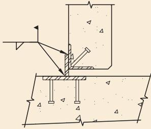
Fig. 4.5.39 Bolted tieback (BTB2).
