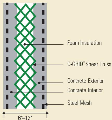
Wall Panel – Shear Truss
